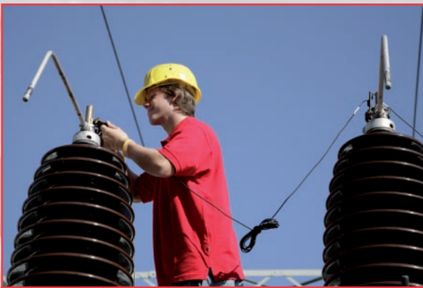
Connecting DIRANA to a bushing
